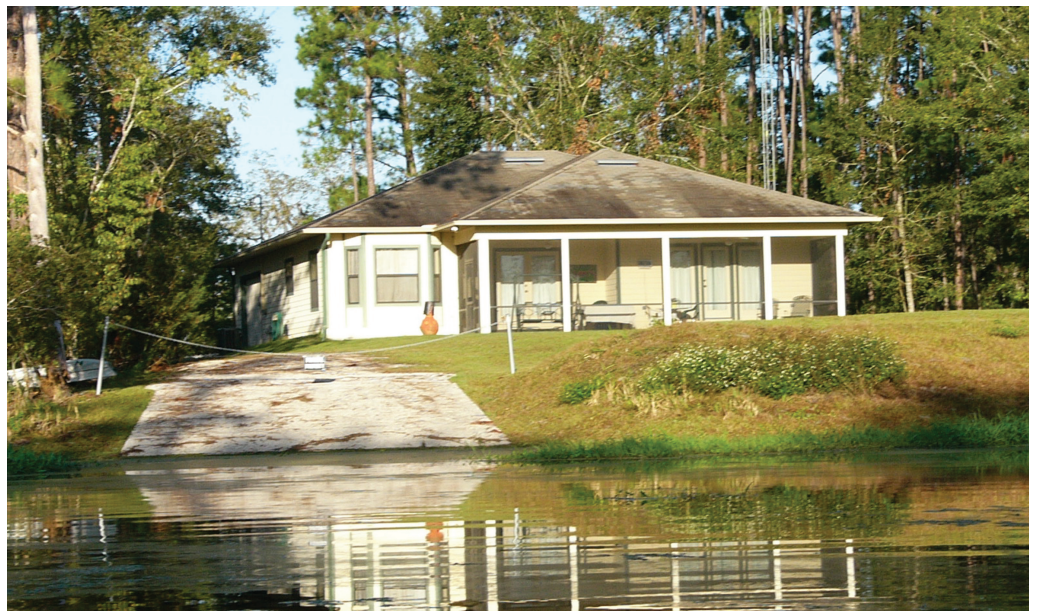
Example of an unhealthy shoreline. No buffer zone between house and waterway. This boat ramp sends runoff directly into the water with none of the filtration provided by a buffer zone.
